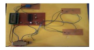
As can be seen from the above circuit diagrams, the rectified voltage from the 4 diodes is given to pin 1 of the respective regulators. Pin 2 of the regulators is connected to ground and pin 3 to Vcc. With adequate heat sinking the regulator can deliver 1A output current. If internal power dissipation becomes too high for the heat sinking provided, the thermal shutdown circuit takes over preventing the IC from overheating.
